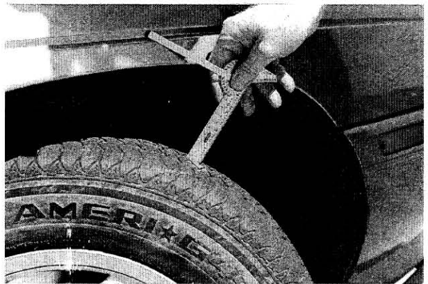
Measuring the depth of tread on a tire. A difference of depth from one edge to another shows misalignment. A different depth of tread between two tires may indicate that the tires are not of the same vintage.
